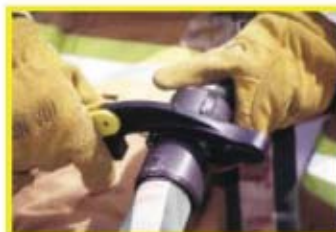
The Res-Q-Rench is designed to work with rocker lug handline and supply line couplings and is the only folding spanner that will work with 4" and 5" storz locking couplings.
