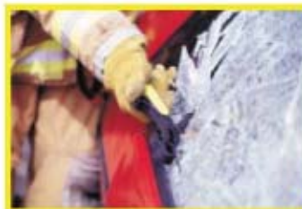
With its integrated carbide tip window punch, the Res-Q-Rench can quickly pop out windows during vehicle extrication.
